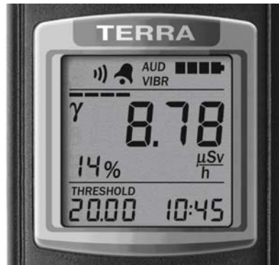
Figure 7 – LCD of the dosimeter (the mode of photon-ionizing radiation DER measurement)
