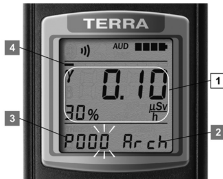
Figure 9 – LCD of the dosimeter (the submode of measurement result saving of photon-ionizing radiation DER)
