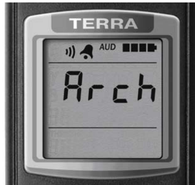
Figure 8 – LCD of the dosimeter (start of the submode of measurement result saving in the nonvolatile memory).
