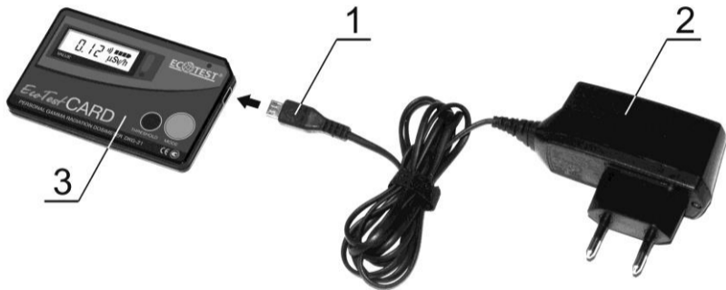
Figure B.3 – Connecting the charger
