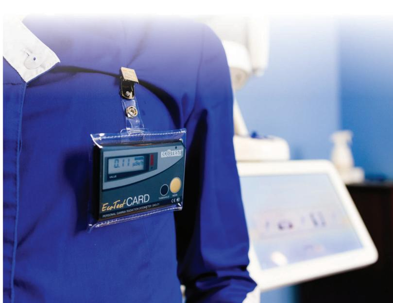
It is possible to set values of threshold levels for dose and dose rate. If the preset threshold levels are exceeded, light and audio alarms are actuated.
