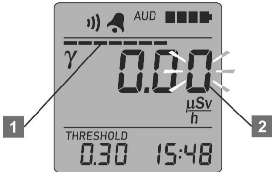
Figure 7 – LCD of the dosimeter (the submode of alarm threshold level programming)
