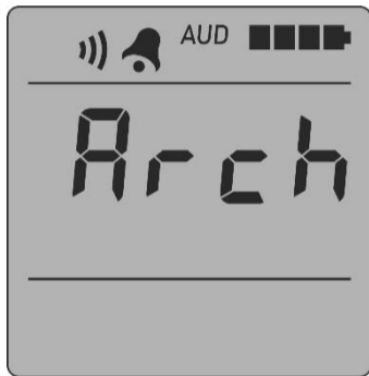
Figure 5 – LCD of the dosimeter (start of the submode of measurement result saving in the nonvolatile memory)
