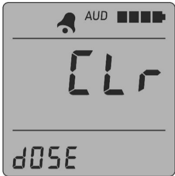
Figure 13 – LCD of the dosimeter (the sumcode of DE and DE accumulation time values resetting)
