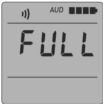
Figure 19 – LCD of the dosimeter (start of the submode of measurement result saving – no free space in the nonvolatile memory)
