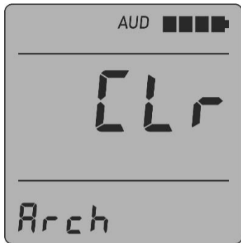
Figure 29 – LCD of the dosimeter (the submode of measurement results clearing stored in the nonvolatile memory)
