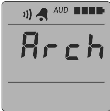
Figure 16 – LCD of the dosimeter (start of the submode of measurement result saving in the nonvolatile memory)
