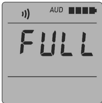
Figure 9 – LCD of the dosimeter (start of the submode of measurement result saving – no free space in the nonvolatile memory)
