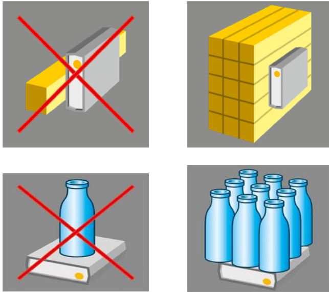
Figure 2.29 – Putting single-type containers together
