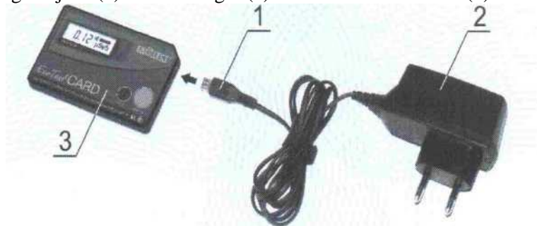
Fig. 4 - Connecting the charger to the dosimeter DKG-21.
