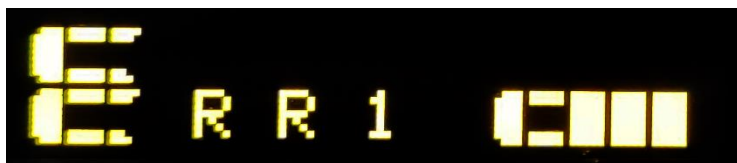
Figure 6 – DER readings display mode when communication with the detecting unit is lost
