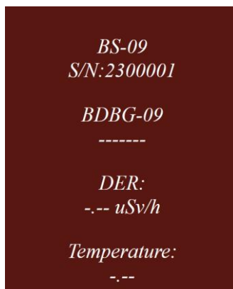
Figure G.6 – Read data (in case of loss of communication with the detecting unit)
