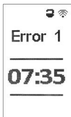
Figure 6 – Displaying a message about the lack of communication with the detecting unit
