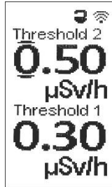
Figure 8 - Mode of changing the threshold levels values
