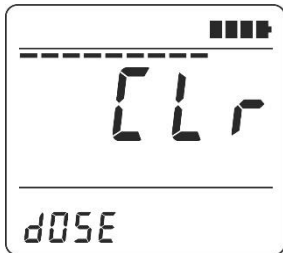
Figure 2.14 - LCD of the radiometer (DE and DE accumulation time reset submode)
