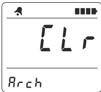
Figure 2.26 – LCD of the radiometer (submode of measurement results clearing stored in the nonvolatile memory)
