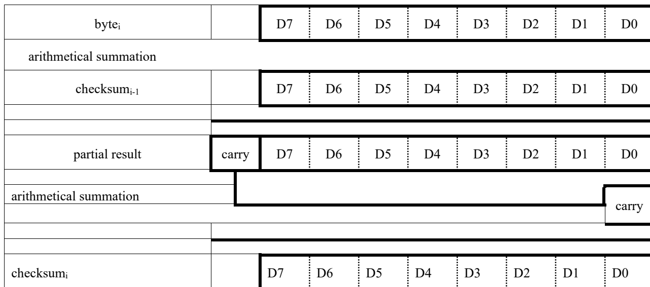
Figure C.1 – Checksum calculation algorithm
