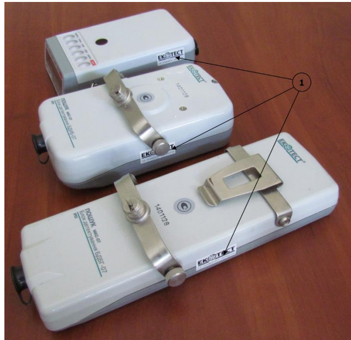
Figure 5 – Example of dosimeter sealing, place marked 1
