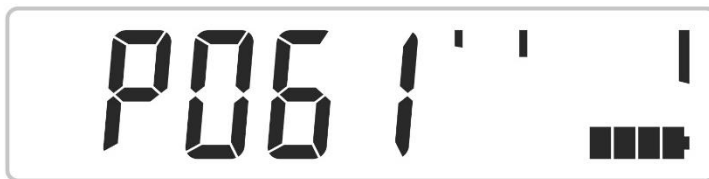
Figure 13 – LCD of the dosimeter (Measurement history viewing, measurement result display)
