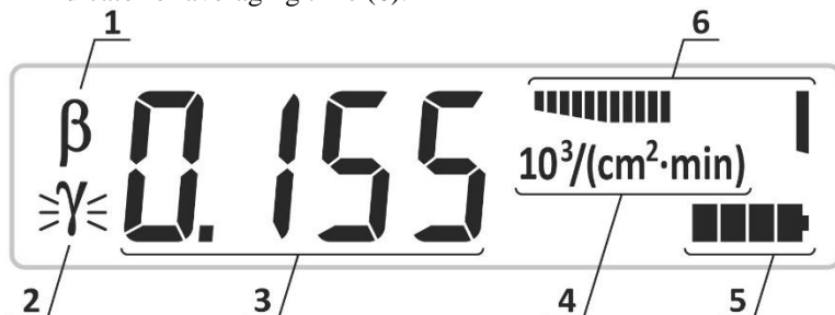
Figure 10 – LCD of the dosimeter (Surface beta particles flux density measurement in precise mode)
