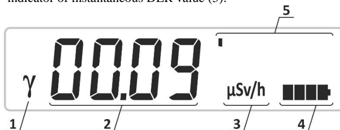
Figure 7 – LCD of the dosimeter (photon ionizing radiation DER measurement in search mode)
