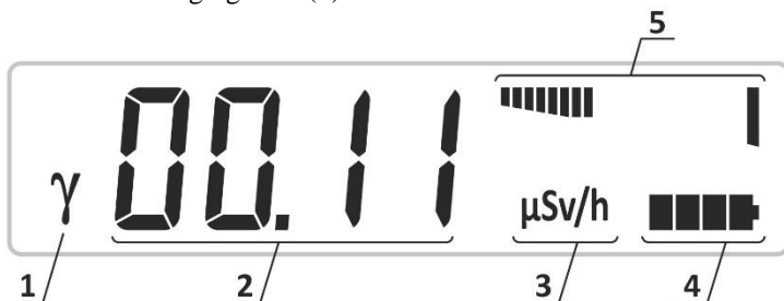
Figure 8 – LCD of the dosimeter (Photon ionizing radiation DER measurement in precise mode)
