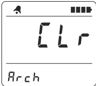
Figure 2.22 – LCD of the radiometer (submode of measurement results clearing stored in the nonvolatile memory)
