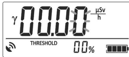
Figure 2.13 – LCD of the dosimeter (submode of the alarm threshold level and the specified limits of statistical deviations programming)
