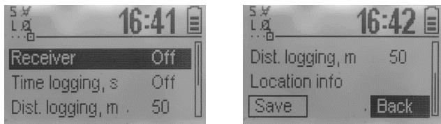
Figure 17 – Setting the parameters of the navigation receiver
