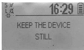
Figure 7 – Gyroscope calibration: holding in a static position
